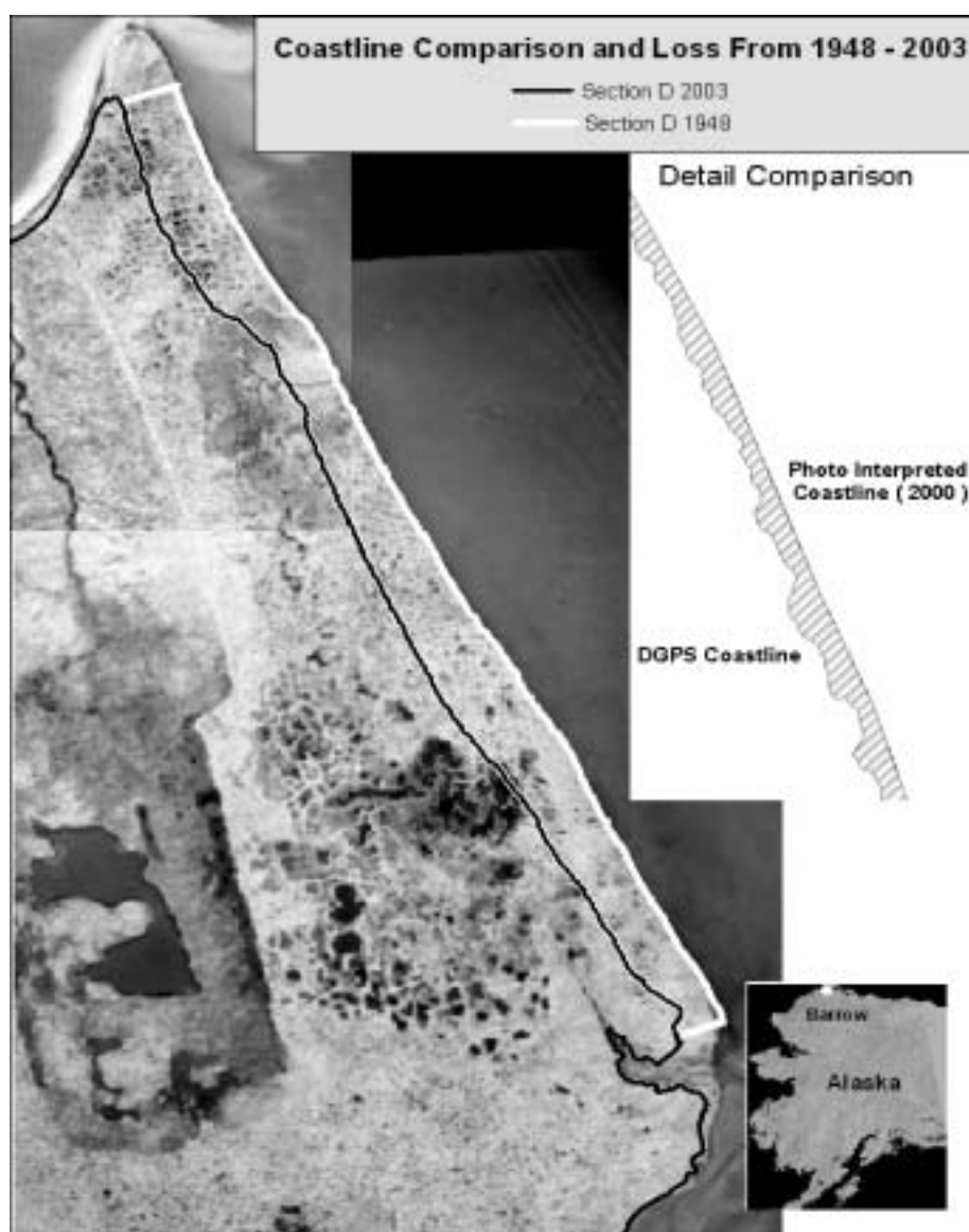
Fig. 1: Comparison of coastline data and detail at zoomed scale, derived from photogrammetric interpretation and DGPS method.
