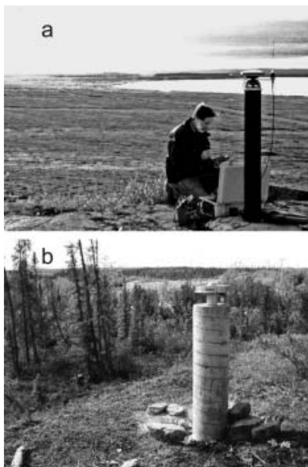
Figure 2. (a) Setting up RTK base station with ground-plane antenna on epoch GPS monument at Kugluktuk NU, August 2002. Insulated stainless steel pillar attached to gabbro outcrop near airport [GKM]. (b) CGPS installation with choke-ring antenna on concrete pillar based in limestone near airport at Inuvik NWT, July 2001 [DLF]. A hemispherical dome has since been added to minimize noise from variable snow load.
